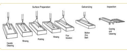
tion having "thick" and "thin" sections welded together will undergo induced thermal stresses (or stress reduction) as the article transits the galvanizing thermal profile from ambient temperature, to ~850°F (~440°C), and back to ambient. For plate girders, the lowest ratio of flange-to web thicknesses possible would be optimum, but in any case, not more than 4:1 if web "oilcanning" is a critical design consideration.
