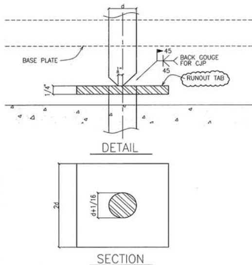
NOTE: CAN TRIM & GRIND RUN OFF TAB AFTER WELDING IF REQ'D.
