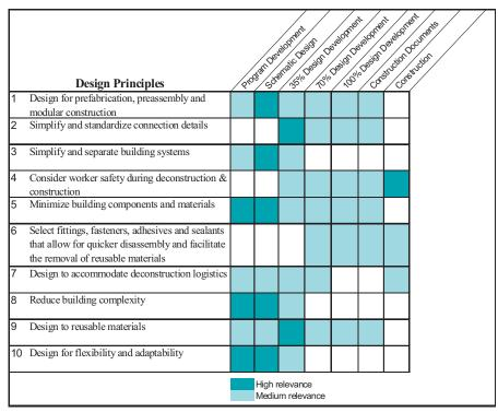
Figure 2. Application Matrix for Design Phases. It identifies the appropriate time to address each principle.
