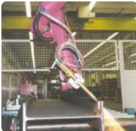
The Kaltenbach KC1200 robotic coping machine (2003 Hot Product Honorable Mention) is one of a number of robotic fabrication machines that recently have been introduced to the steel-fabrication industry. Jesse Engineering's Robotic Series SHC-BC-R (next page) also uses a robot to precision-cut structural steel members.
