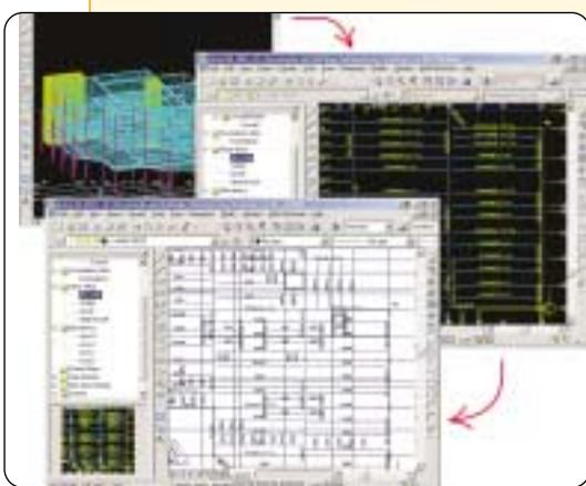
The engineer first creates a RAM Structural System model and imports it into RAM CADstudio for preliminary drawing creation. The CAD specialist can update the drawings, adding details, making partial plans, placing text in the desired locations, and more, with CADstudio's advanced file navigator and drag-and-drop capabilities. The drawings can be modified using standard AutoCAD commands and custom LISP routines.
