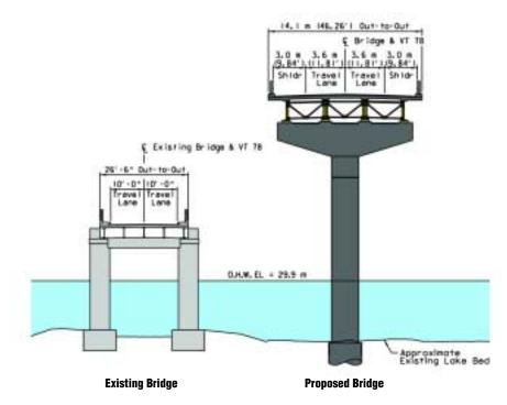
The higher vertical clearance of the proposed bridge eliminates the need for a bascule drawbridge at the center of the span.
