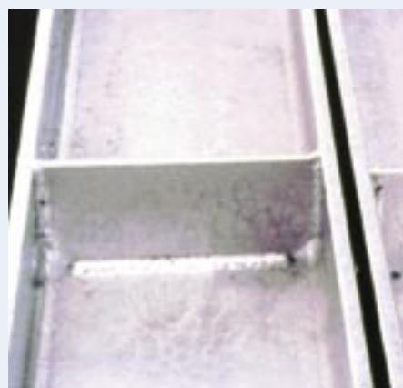
Cropped corners allow molten zinc to flow in and out of tight spaces, avoiding "pooling" in these areas causing excessively thick coatings that may flake during rough handling.
