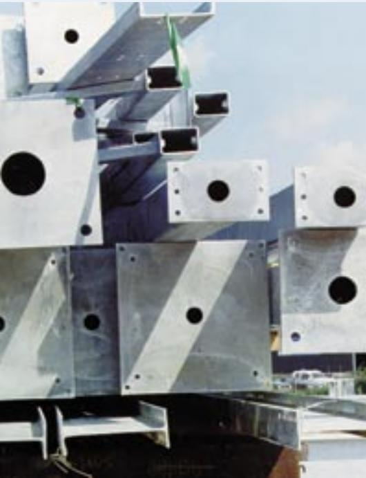
Vent and drain holes prevent trapped moisture or gas from flashing to steam in the heated galvanizing kettle, which may result in localized uncoated surfaces or ruptured fabrications.
