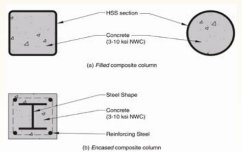
Chapter I of the 2005 Specification covers the design of concrete filled HSS columns and encased composite columns. ratio decreased below 4% and the designer was required to use the provisions of ACI 318, *Building Code Requirements for Structural Concrete and Commentary*. All concrete and reinforcing steel detailing requirements for encased composite columns must conform to the applicable building code, which normally references ACI 318.
