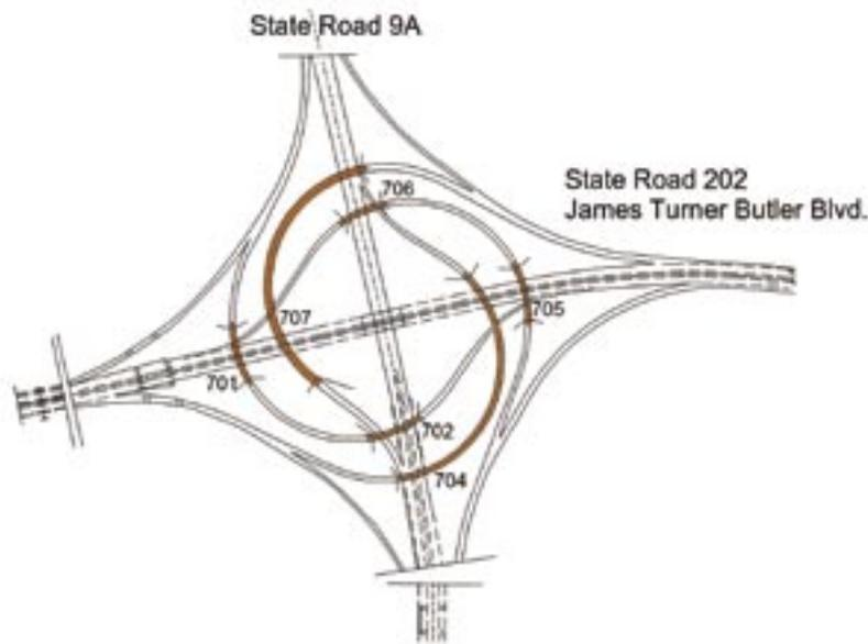
**A steel design saved the Florida Department of Transportation 10 percent—nearly \$8 million—in the final bids for a six-bridge interchange now under construction in Jacksonville, Fla.**
