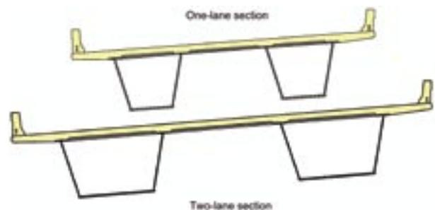
Bridge superstructures consist of double trapezoidal box girders. Following NSBA recommendations, all top and bottom flanges of a box girder will have a common width. Increased flange thickness, rather than width, will accommodate the need for greater support.
