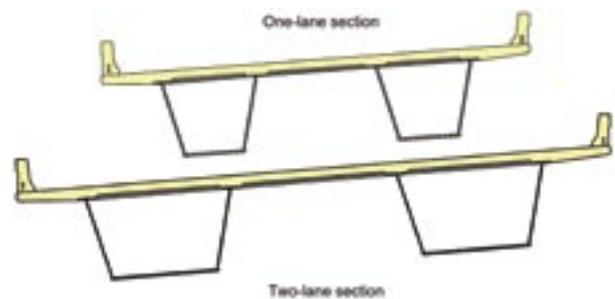
Bridge superstructures consist of double trapezoidal box girders. Following NSBA recommendations, all top and bottom flanges of a box girder will have a common width. Increased flange thickness, rather than width, will accommodate the need for greater support.
