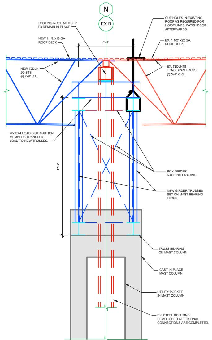
Section A-A through twin girder trusses.
