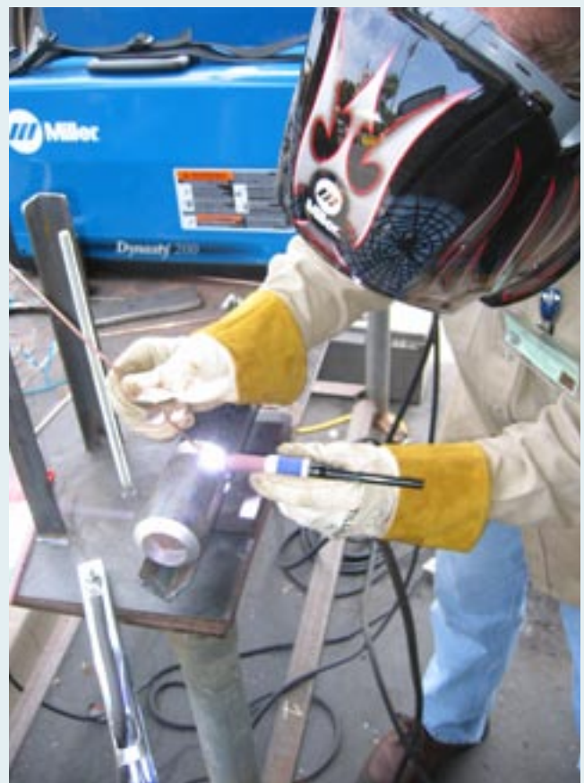
A Miller district manager demonstrates TIG techniques using a Dynasty 200 DX, an inverter power source with advanced Square-wave, Auto-Line, and Lift-Arc technologies.
