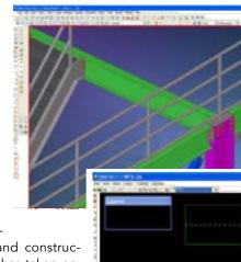
sign to detailing and construction. The company has taken on layout and outfitting, the most expensive shop fabrication operation. The result is a program that allows CNC information to be read directly from the Tekla Structures 3D model to the fab-
