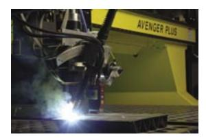
ciency and superior gap tolerance, the HLAW can be installed into many types of equipment, including 2D gantry welding systems, 3D robotic systems, and custom automated systems. A far sturdier tool, HLAW features faster welding speeds, slower cooling rates, and a low heat input that reduces plate distortion.
