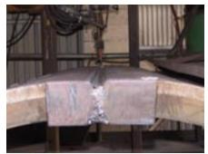
The cylinders required about 30 passes for the inside weld and about 30 passes for the outside weld.
