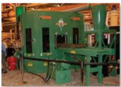
copes and flange thinning; process all interior web/flange cuts for building electrical, heating, ventilation, etc.; and provide part identification to replace laborious shop layout. All of this is available in a compact design that requires a small shop footprint.
