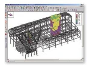
model (pictured) that took 11 minutes and required over 600 MB of space to solve using industry standard technology, solves in 6 seconds and requires only 2 MB of space using Version 7. While this new technology is an "under the hood" improvement, it is quite significant in that it makes practical the solution of much larger and more complete models, as well as greatly increases the design engineer's ability to test different scenarios. This usually results in better designs.
