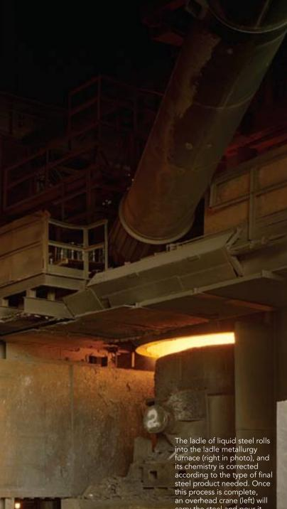
this process is complete, an overhead crane (left) will carry the steel and pour it into the continuous caster for forming into rough beams.
