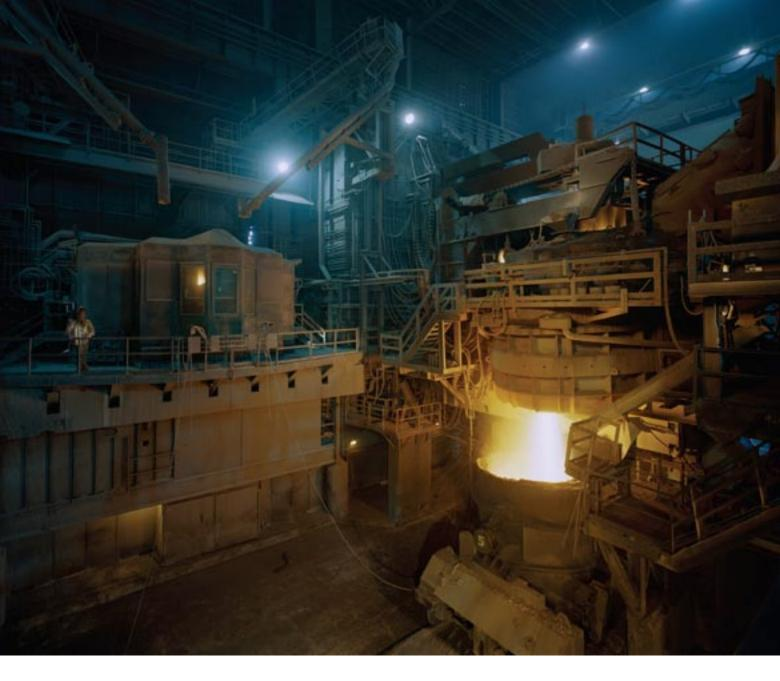
Once the steel is melted to about 3,000 °F and is ready for refining, it is "tapped" from the furnace down to a vessel called a ladle before being taken to the ladle metallurgy furnace. Employees in the control room, or tapping pulpit (at left), monitor the process.
