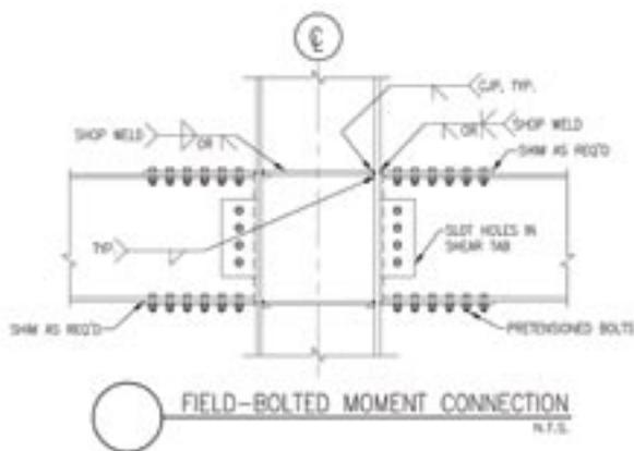
Figure 2. Typical field-bolted moment connection detail.
