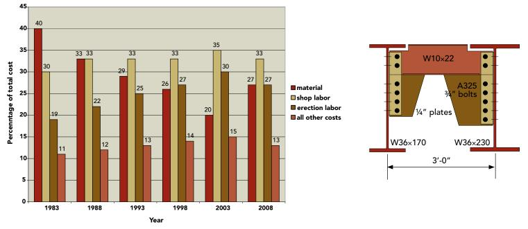
Figure 1. Material, shop labor, erection labor, and other costs—1983 through 2008.
