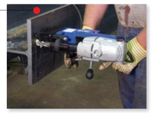
The drill weighs just 30.5 lb and measures  $16\frac{3}{4}$  in. x  $7\frac{3}{16}$  in. x  $8\frac{14}{4}$  in. long, yet provides drilling capacities of from 7/16 in. up to  $1\frac{1}{2}$  in. diameter and a 2-in. depth of cut. For versatility, the drill also includes Hougen's new hex drive arbor, which can be easily removed for installation of drill chucks and other Hougen Portable Machine Shop accessories.
