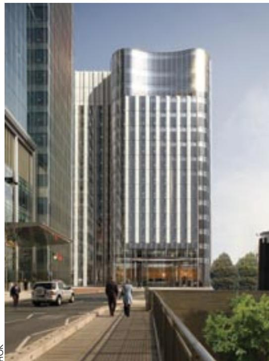
**Opposite and above:** The building's cladding panels will be top hung and fixed off of channel inserts into the concrete floor slab.
