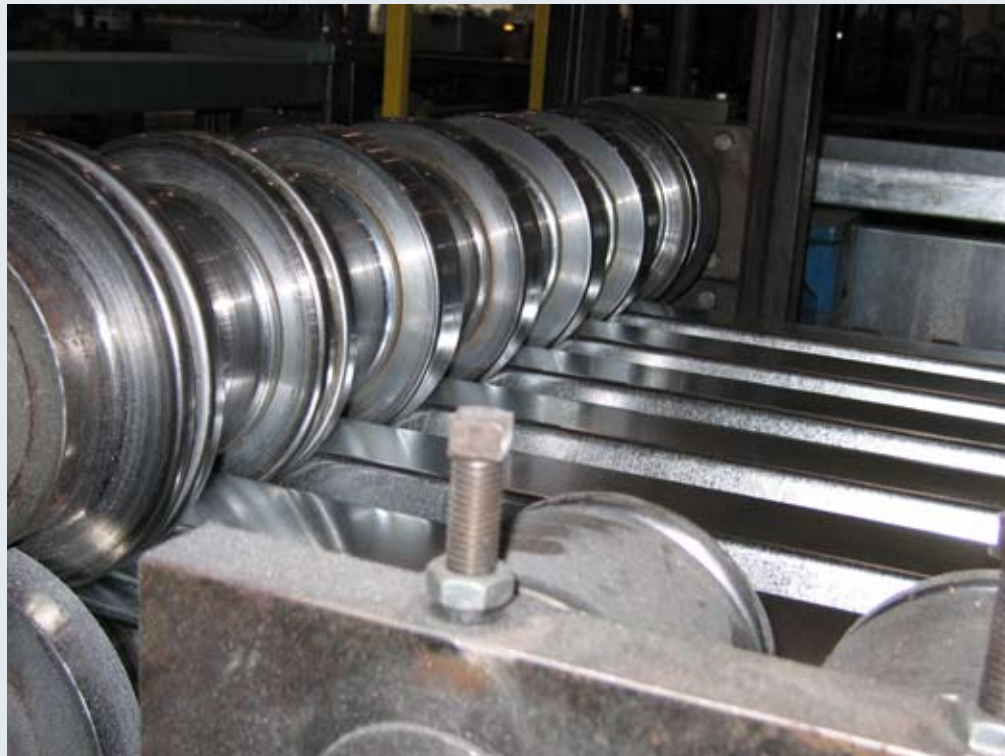
Steel deck being formed, with flutes being created from the center out.
