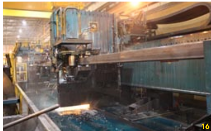
The saw attaches to the tube and cuts individual sections.
