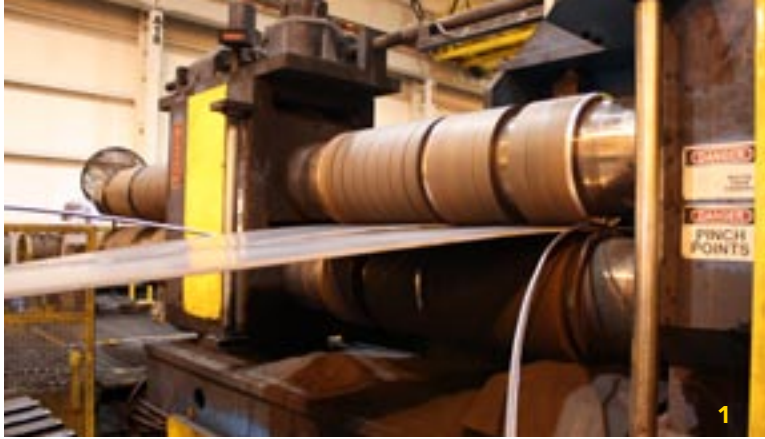
The slitter, creating two new widths of steel; sheared scrap (right) is recycled.
