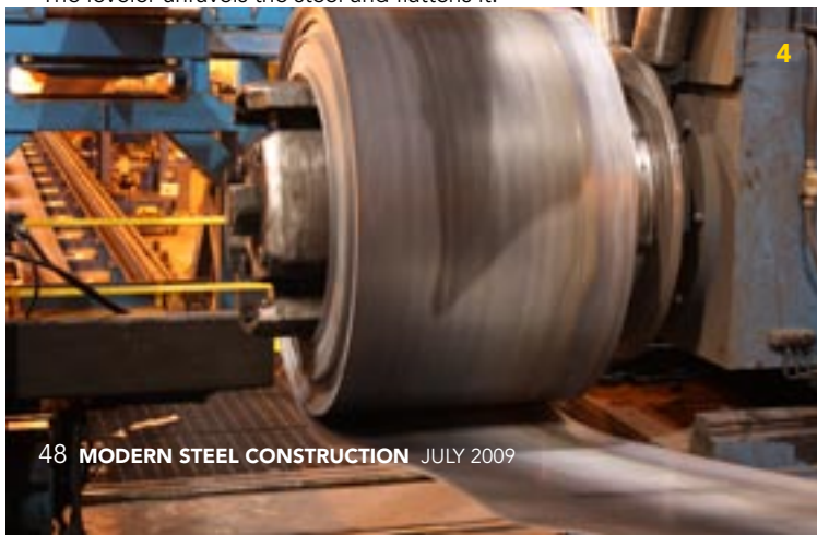
The leveler unravels the steel and flattens it.
