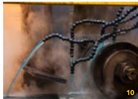
Steel is lubricated throughout the production line.
