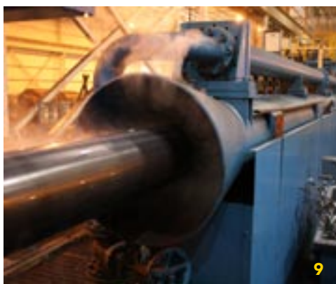
Newly formed tube enters the cooling trough before being cut or formed into a rectangular shape.
