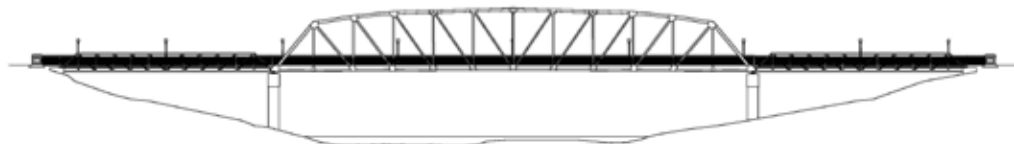
In 2008 the bridge was reconstructed. One truss span was lengthened to 222 ft using parts from the second truss as well as new components, and new approach spans were added.
