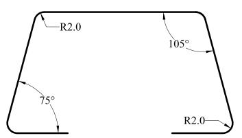
**Fig. 1** Typical cross section for the Folded Plate Bridge System. Dimensions vary based on span length.
