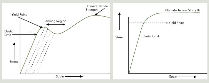
Plastic bending takes place in the zone marked "Bending Region." The dotted lines show how the material will spring back when the bending load is removed. The spring back reduces as the strain is increased.
