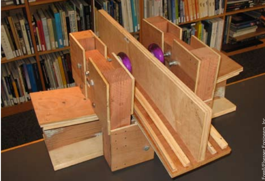
Above: The team bought into the concept of the uplift restraint devices after Forell/Elsesser's Mason Walters, S.E., built a 1/3-scale model using wood and roller blade wheels. The vertical restraint is only activated by an uplift force and still allows unimpeded horizontal movement.
