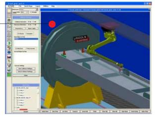
including cutting, coping, layout marking and welding. Using these systems, the fabrication of each individual part can be fully programmed from start to finish. These solutions will provide the structural steel fabrication industry with unprecedented automated programming and fabrication capability.
