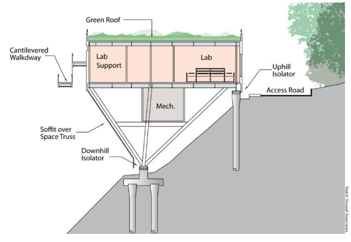
A typical section of the RMB shows the split-level base isolation system and the steepness of the hillside below.
