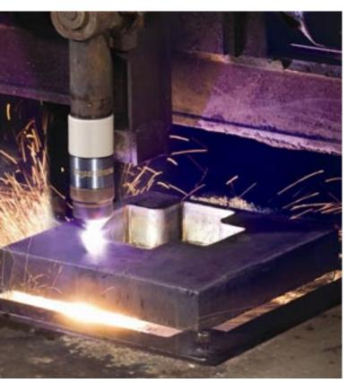
Keeping the shield cool on a plasma torch can dramatically reduce the amount of slag build-up, reducing maintenance requirements and extending equipment life.
