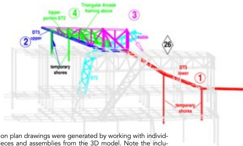
Erection plan drawings were generated by working with individual pieces and assemblies from the 3D model. Note the inclusion of temporary shores and cable attachment requirements.
