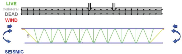
These diagrams show a few of the many common load combinations that would have to be assembled from all of the applied load categories (not comprehensive).
