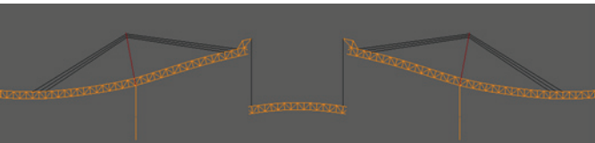
Figure 8: The cables are stressed in one step, but do not at that point take up the camber in the span adjacent to the main span.
