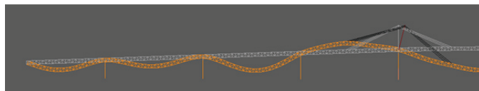
Figure 2: Unbalanced system with dead load and cable tensioning applied.
