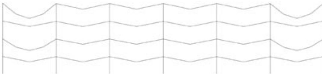
Deflection With Staggered Double-Span Framing
