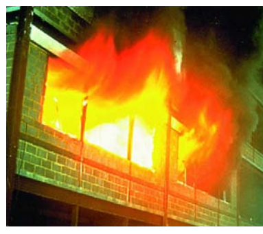
1998: The Cardington fire tests encourage designers to contemplate performance-based fire design as a practical alternative to prescriptive designs.
