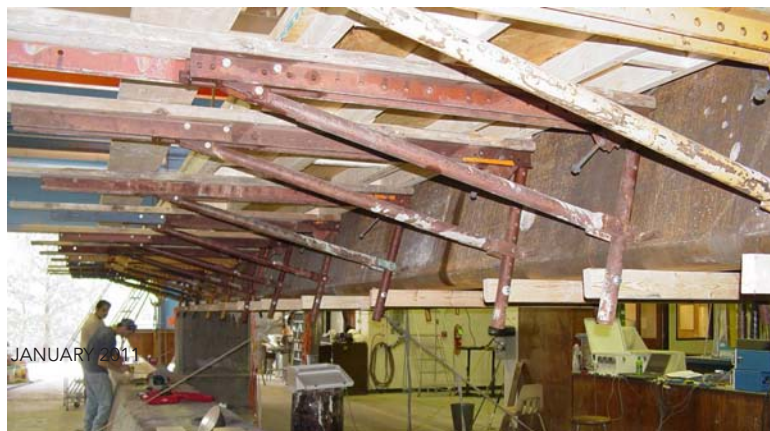
2009: Folded plate girder bridge systems have the potential to revolutionize the short-span bridge market.
