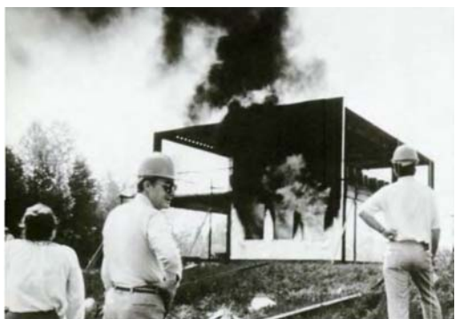
1983: National Bureau of Standards and AISI conduct tests that confirm the accuracy of FASBUS II fire computer modeling.
