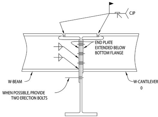
▲ **Fig. 6:** Cantilever Moment Connection at W-Beam when End Moment is not Reversible (Bottom Flange is Always in Compression)
