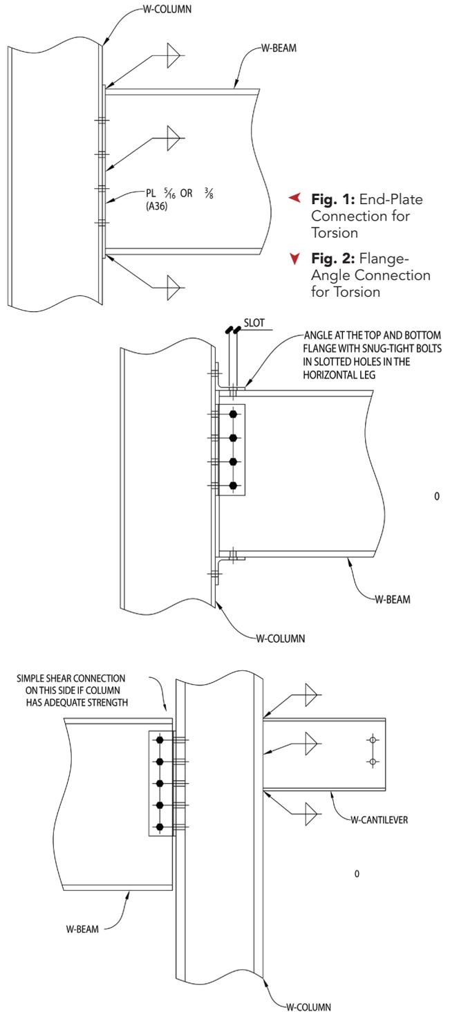
▲ Fig. 3: Shop Welded Short Cantilever
