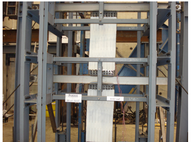
▼ Fig. 2: Two-story SSPF specimen at 2% drift.
