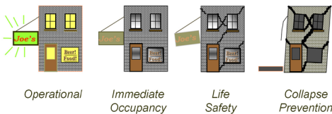
▲ Fig. 2: The ASCE 41 performance levels: Operational, Immediate Occupancy, Life Safety and Collapse Prevention.
