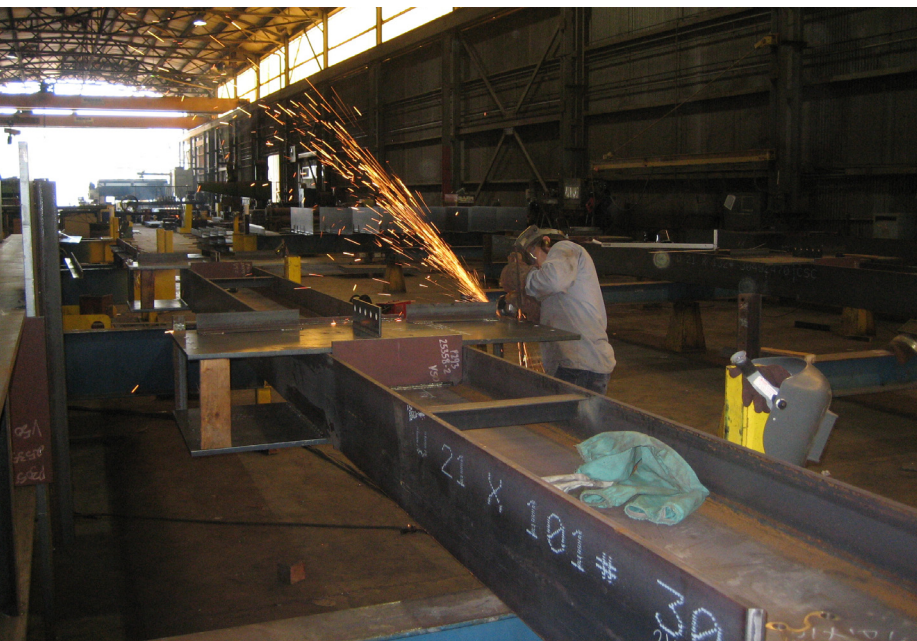
▲ Preparing a column in the SteelFab shop. In addition to keeping all the welding in the shop, attaching the plates requires only fillet welds, which simplifies both welding and inspection.
