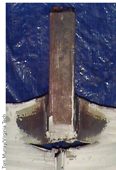
▼ Fig. 4: Tension rupture of Whitmore section.
