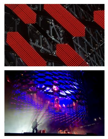
▲ A dynamic steel frame designed by Buro Happold engineers enabled the 3,800-sq.-ft video screen to rapidly expand to 73 ft height, taking its place as the centerpiece for the U2 360° Tour.
