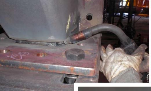
Using the proper size nozzle and shape can help welders gain better joint access and with it improved shielding gas coverage to prevent issues like porosity. A flexible neck torch can also help maneuver into difficult joints.
