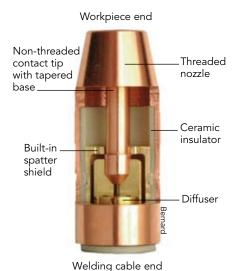
A This cutaway view of Bernard's Centerfire MIG gun consumables shows the various components that contribute to better gas coverage, longer tip life and better arc starts.
