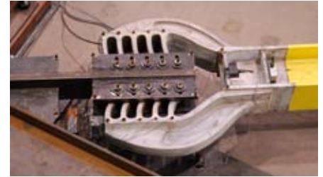
▲ The full-scale test frame at the University of Toronto with the Scorpion brace in the neutral position. A short video of the frame being tested aired on the Discovery Channel and can be viewed at http://bit.ly/gvji3U .
