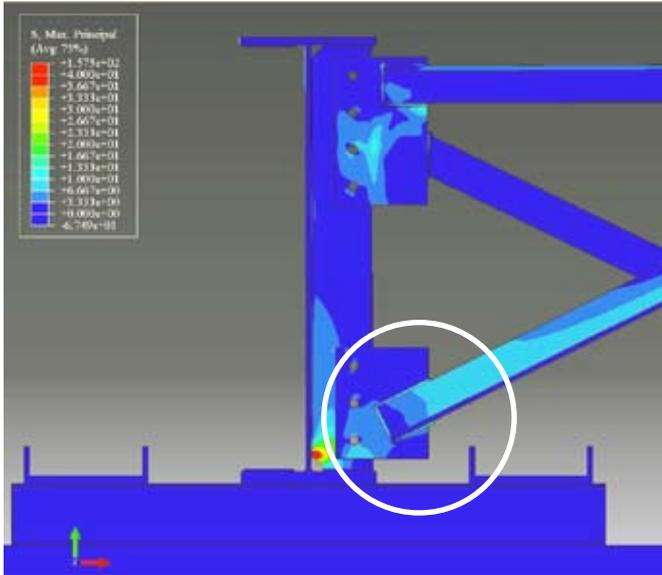
▲ Fig. 3: Cross-sectional view of unretrofitted specimen, with web gap shown in circle.
