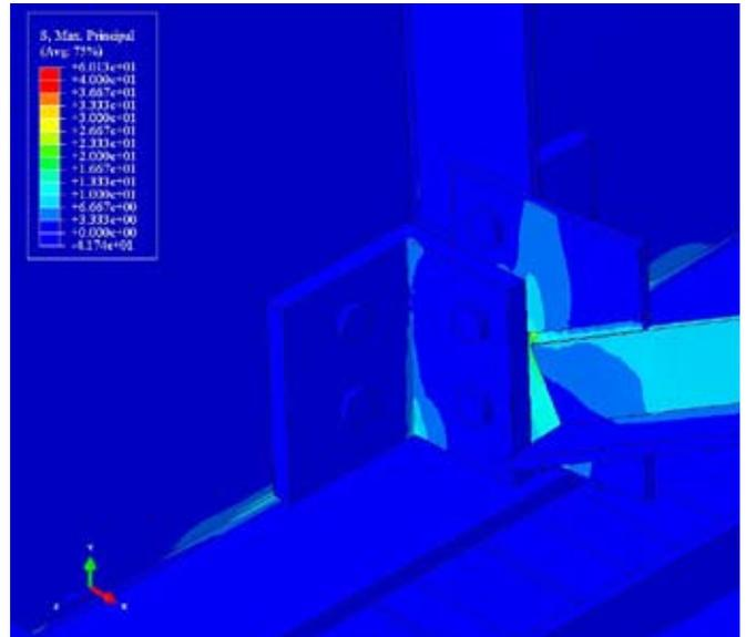
▲ Fig. 4: Interior side of girder shown with bolted angles connecting the web to the stiffener.
