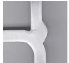
▲ Fig. 1: An illustrated (a) and macro-etched (b) CJP joint between round HSS and a Cast ConneX High-Strength Connector.
