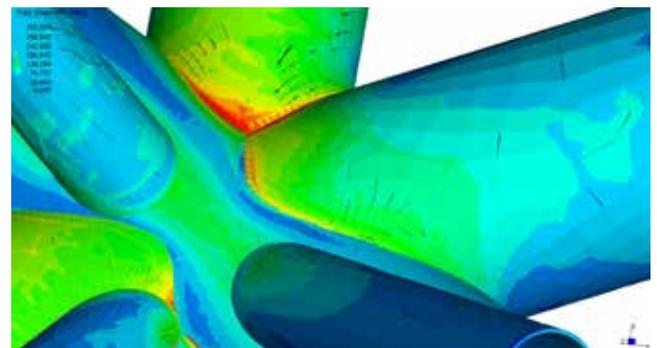
▲ FEA post-processing, indicating the stress contours of an HSS node.
