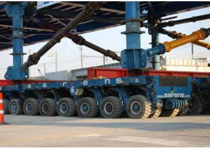
▲ Rolling in the 394-ft-long, 2,375-ton steel truss railroad bridge on SPMTs.
