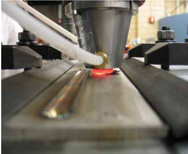
▲ Weld setup and pin tool during the FSW process.
