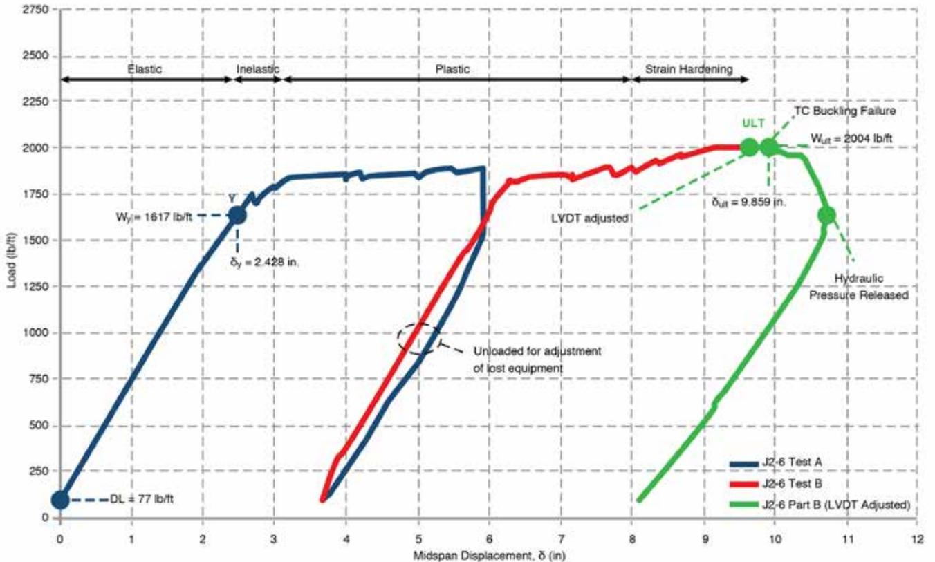
▲ During an overload, the primary limit state established by the Flex-Joist system is characterized by prolonged phases of deflection, moving from the initial elastic phase through to strain hardening, followed by a loss of load-bearing strength, buckling and collapse.
