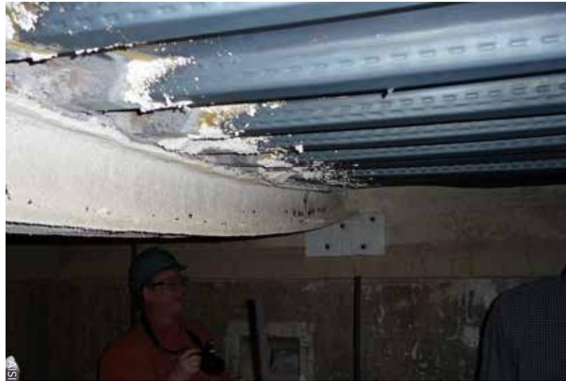
▲ ► An unrestrained steel-framed floor specimen, before and after the fire test.
