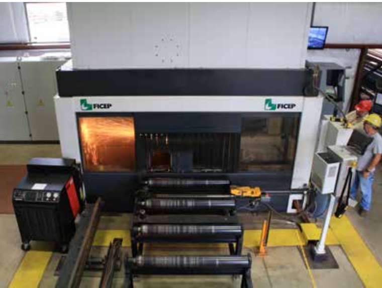
▲ The coping machine, one component of the company's fabrication processing system.
