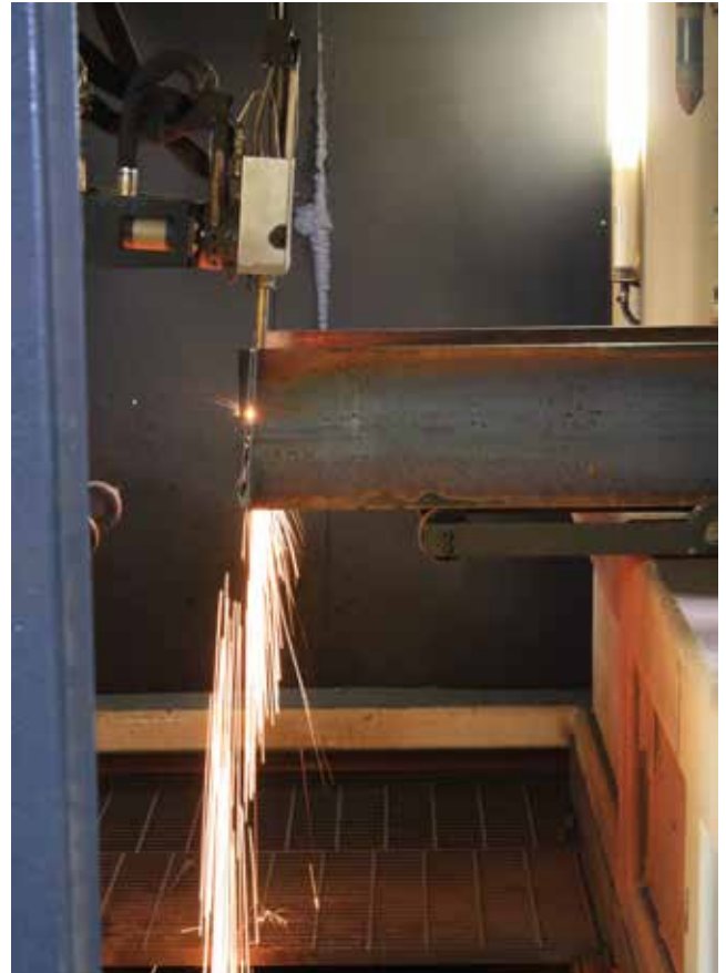
▲ The coping machine, which performs both oxy and plasma cutting.
