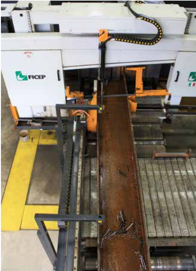
▲ Dave Steel's Ficep saw. The company plans to install a smaller saw as well so as not to tie up the main saw with smaller jobs.
