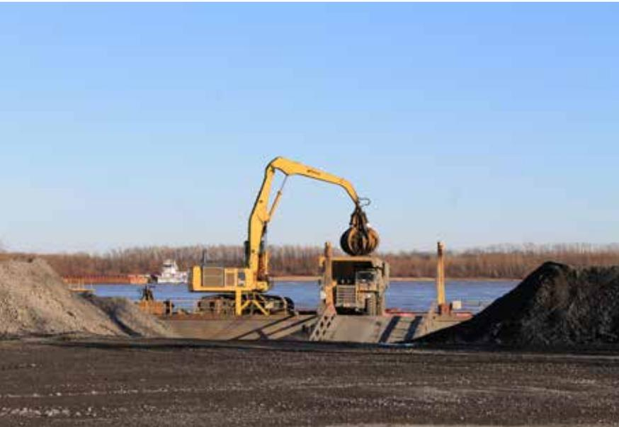
▼ Scrap is separated into multiple types. A consistent “recipe” of steel from the various piles is used to create the products.
