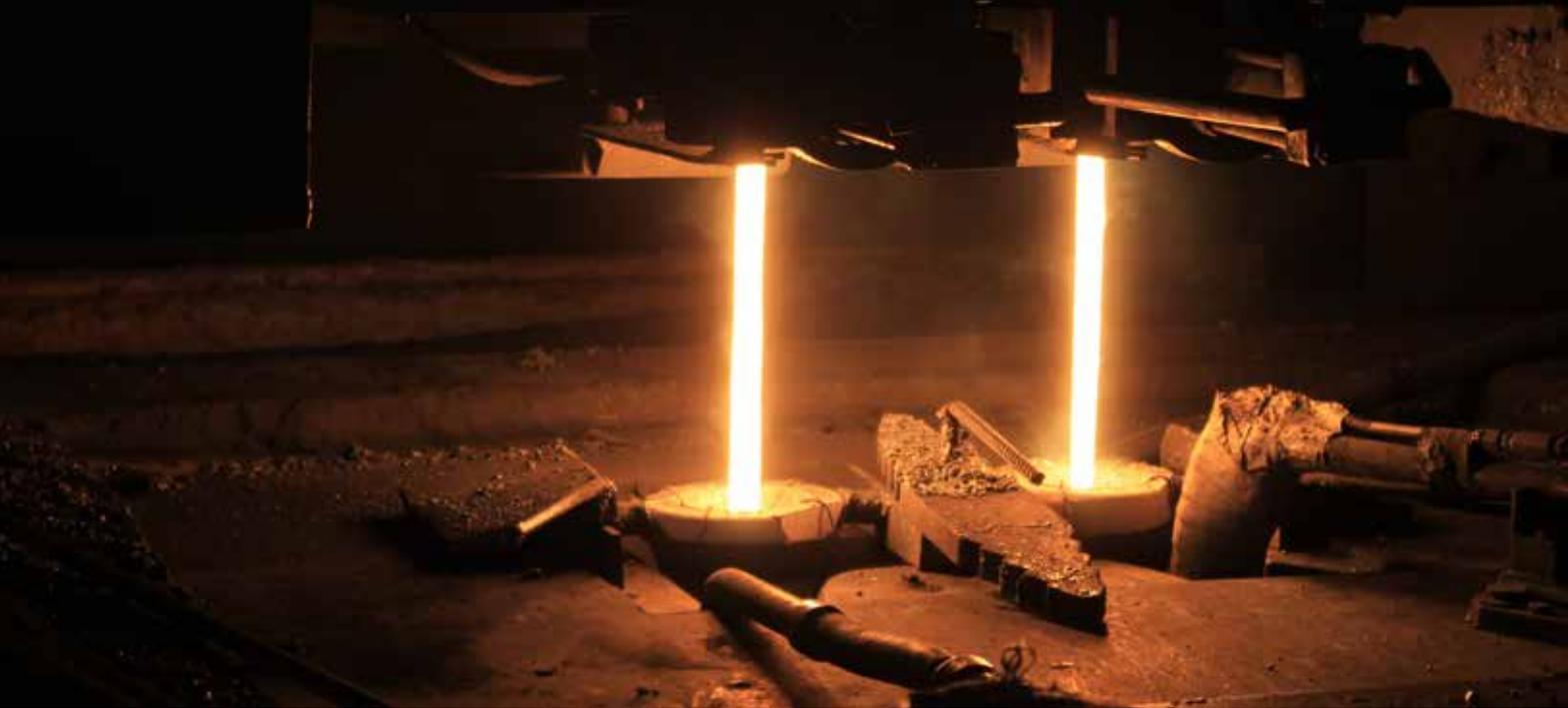
▲ Casting the steel. Two molten steel streams are fed into molds. Granulated powder is also continuously fed into the molds so that the steel doesn't stick—much like greasing a pan.
