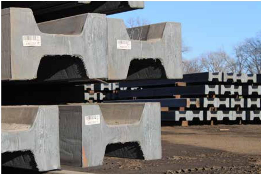
➤ After cooling, beam blanks are often stored outside before they are ready to be reheated and rolled into shape.
