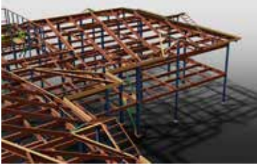
◀ Structural steel was used for roof framing.
